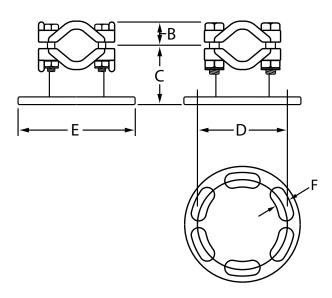
Type "D" is a line of rangetaking bus supports for cable. It is available for cable O.D.'s from 36" to 2%". These units can also be used for rod and tubing bus.
